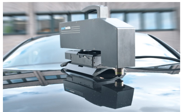
Fig. 2 The optical 3D surface inspection is ideal both for the lab as well as demanding industrial use, e.g. for checking paint appearance in the automotive industry (Image: NanoFocus)
